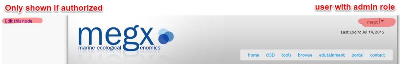
Figure 5: Special content is only shown if user is authorized. Here, the user 'megx' is in role admin and therefore a link is displayed on the top-left to edit the content of this page.
